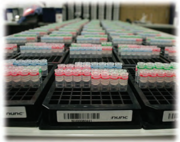
The Healthy Ageing BioBank team stores blood and urine samples in tiny cryovials (tubes) at -170^{\circ}\text{C}
